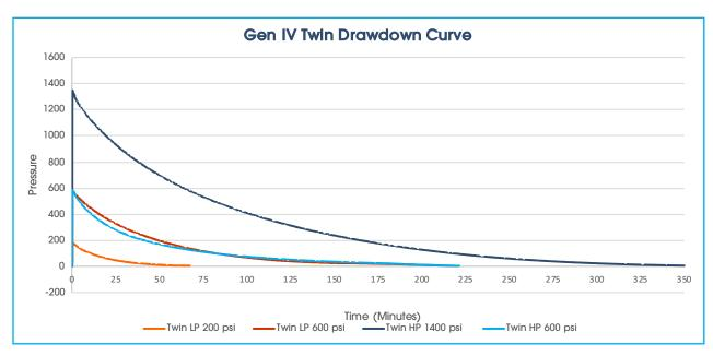
NOTE: Air supply for each test was the same: 700 cfm at 150 psig. Results can vary depending on many factors including air compressor, temperature, hose length, etc.
