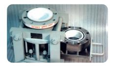
The ONIS Quick-Action Rupture Disk Changer is designed to optimize disk replacement.
