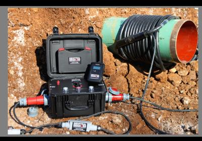
The IDMAG Pipeline Demagnetizer System can be used on virtually any size pipe to remove magnetism and eliminate arc blow and other issues.
