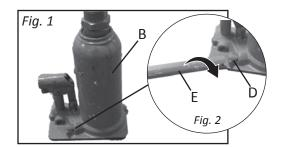
**1.** Release all pressure from hydraulic cylinder (*B*, *Fig. 1*) by turning release valve. (D, Fig. 2)
