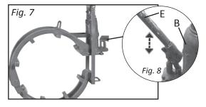
**6.** Close clamp by pumping the hydraulic cylinder (B) upwards. (Fig 7)
