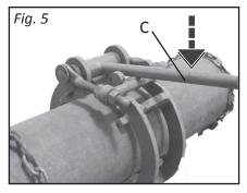
**1.** Lift hand lever (C) to release the hand lock placement (A) free from holding ears. (D, Fig. 1)
