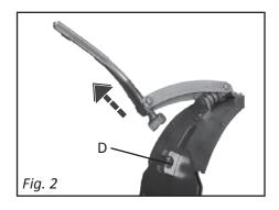
**2.** Release band from latch base assembly. (D, Fig. 2)
