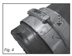
**4.** Close band by pushing down latch handle. (C, Fig. 4)
