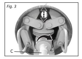
. Turn crank handle (C) until pipe has formed back to its round shape. (Fig. 3)
