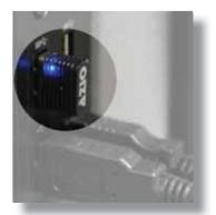
If your PC or laptop does not have builtin Bluetooth, insert a Bluetooth adapter ("dongle") into its USB as shown here.
