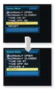
RESET deactivates a triggered relay. (It does not change relay settings.)
