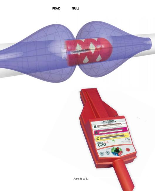
As you move the antenna closer to the pig, the signal strength increases until you reach the peak, then drops to little or no signal as you approach the signal null point.
