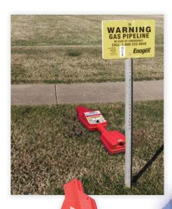
The TRAXALL may be positioned directly onto an exposed pipeline. (Note molded shape on case bottom to aid alignment.)
