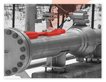
Once a passage has been detected, the LED array will light up. Here, the TRAXALL 620 indicates a pig configured with a 27.3 Hz transmitter has arrived.
