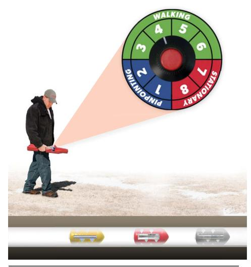
Here, the operator is approaching three pigs in close proximity to each other and configured with active transmitters. LED arrays are independent of each other and each will light up according to relative signal strength as approached.
