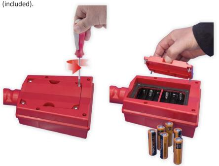
Insert six AA-cell alkaline batteries (also included). Observe battery polarity as shown on receptacle. Check seal for deformation, cracks, tears, or foreign objects. Replace cover. Tighten screws carefully and evenly to maintain a weatherproof seal. DO NOT OVERTIGHTEN.
