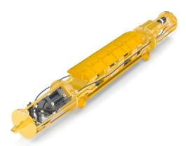
Length 107" (2718) Width 12" (305mm) Height 16" (406mm) Weight 930 lbs (421 Kg) .9 hp - Cooper Air Motor Cylinder 6" (152mm) 180-210psi Working Air Pressure Pipe Size Range 16" (406mm)
