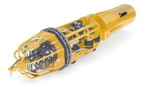
46"-48" (1167-1219mm) Pipe Size Range Wall Thickness Range .375"-.750" (9.5-19mm) Standard Length 148" (3759mm) 42" (914mm) Width 42" (914mm) Height Weight 3700 lbs (1678 kg) Working Air Pressure 200-220 psi Air Motor (2) 2.7 hp Drive Motors - Side Drive Air Tank 80gal w/ 4.7 gal reserve Clamping Shoes 48 total clamp shoes, 24 on each section Cylinder 14" (356mm) Climbing Capability 25° + slope
