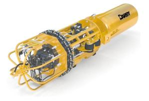
34"-36" (864-914mm) Pipe Size Range Wall Thickness Range .375"-.750" (9.5-19mm) Standard Length 145" (3686mm) 31" (787mm) Width 31" (787mm) Height Weight 2715 lbs (1232 kg) Working Air Pressure 180-220 psi Air Motor (2) 2.7 hp Drive Motors Air Tank 80gal w/ 1.6 gal reserve Clamping Shoes 36 total clamp shoes, 18 on each section Cylinder 12" (305mm) Climbing Capability 25° + slope
