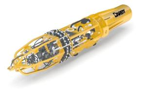
Pipe Size Range 20"-22" (508-559mm) Wall Thickness Range .125"-.500" (3.18-12.7mm) on 20"(508mm) .125"-.750" (3.175-19.05mm) on 22"(559mm) Standard Length 114" (2896mm) Width 18" (457mm) Height 18" (457mm) Weight 810 lbs (367 kg) Working Air Pressure 180-220 psi Air Motor .9 hp Cleco Air Tank 15 gal w/ 3 gal reserve Clamping Shoes 20 total clamp shoes, 10 on each section Cylinder 8" (203mm) 25° + slope Climbing Capability
