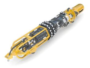
Pipe Size Range 10" (254mm) Wall Thickness Range .125"-.5" (3.18-12.7mm) Standard Length 68" (1727.2mm) Width 10" (254mm) Height 10"(254mm) Weight 235 lbs (107 kg) Working Air Pressure 180-220 psi Air Motor Non Powered Air Tank 2 gal **Clamping Shoes** 15 total clamp shoes, 12 shoes at the joint (6 on each section) 3 shoes on rear section Cylinder 6" (152mm) Climbing Capability N/A
